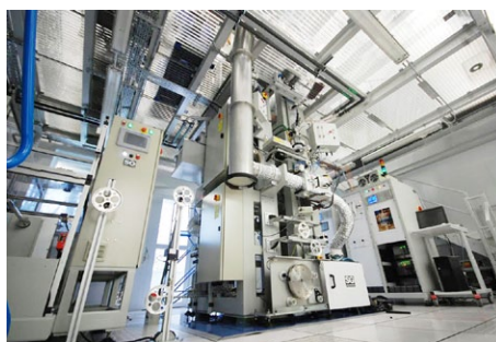
Silica fibre drawing tower in the Zepler Institute cleanroom complex.
